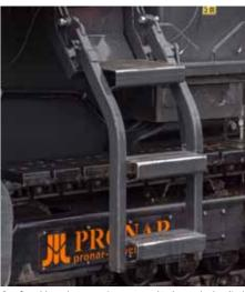
Comfortable and ergonomic entrance thanks to a hydraulically foldable ladder
