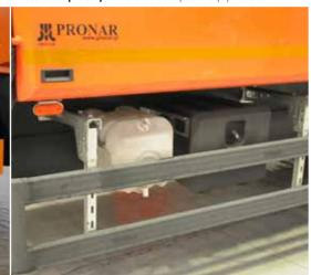
**Side-guards protection system** stops the machine when side shields are opened by unauthorized personel
