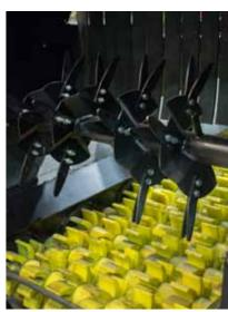
Starscreen can be used instead of trommel. Utilising starscreen during works on wet material increases machine efficiency. The rotation speed of the stars can be steplessly regulated which allows for accurate setting of the separated fraction
