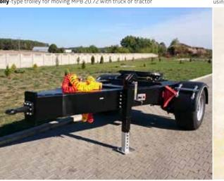
**Ball coupling** enables repositioning of the trommel screen using construction machinery
