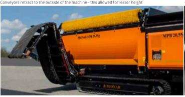
Tracked chassis for moving the machine without any additional towing
