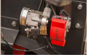
Central system for exchange of operating fluids has been placed on the left and right sides of the machine
